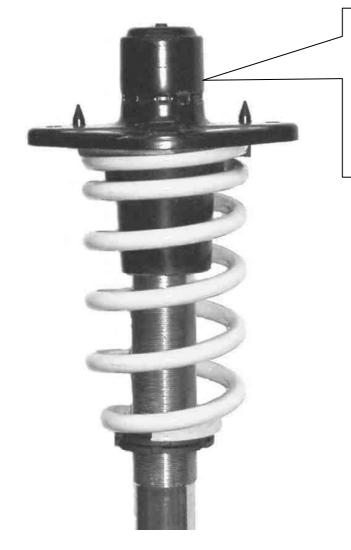
Put on the original supporting bearing, bump stop and dust cover. Tightening torque for the piston rod is 25 Nm (18 ft-lb). Please install the strut unit to manufacturers recommended settings regarding tightening torque and fixing specifications.
