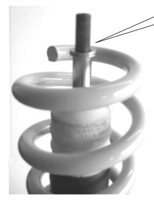
Adapt the original top mount onto the strut and fix it with the supplied nut. Tightening torque for the piston rod is 40 Nm (29 ft-lb). Please install the strut unit to manufacturers recommended settings regarding tightening torque and fixing specifications.
