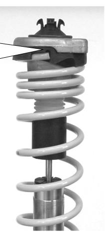
The wide overlaying side of the fixing eye has to be mounted towards the wheel.
