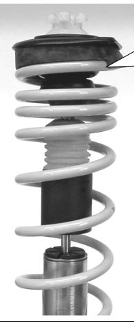
The supporting bearing has to be mounted with all parts as on the standard kit. Tightening torque for the piston rod is 25 Nm (18 ft-lb). Please install the strut unit according to manufacturers recommended settings regarding tightening torque and fixing specifications.
